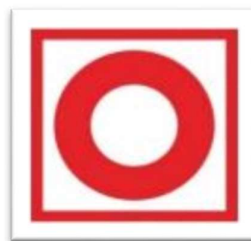
ROP – manual start up alarm bells
